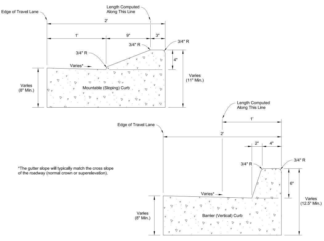
Figure 5-07: Typical Curb and Gutter Shapes and Dimensions
